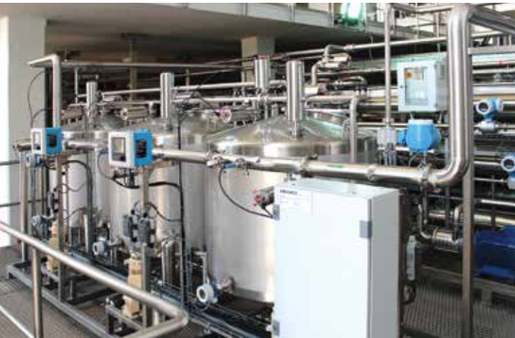
An electrodeionisation plant, 5 x 100 m 3 /h
