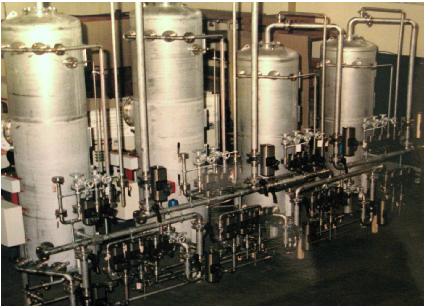
THE FERTAREX SHORT- CYCLE UP- FLOW COMPACTED RESIN BED ION - EXCHANGE SYSTEM WITH INTERNAL REGENERATION AT THE FERTILISER COMPLEX PETI NITROGEN - HUNGARY START UP 1987
